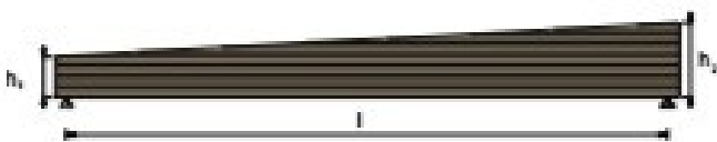
Double tapered beam with straight lower chord
